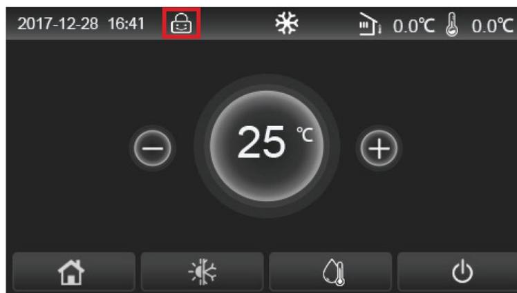
In this condition, the touch functions of the display are disabled. Pressing
