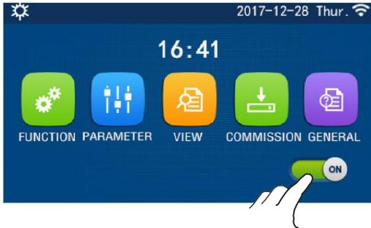
Fig. 3: Turning ON
