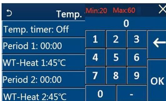
By clicking on the labels relating to the flow temperature parameters, a numerical screen will appear on the right side (with indication of the range of allowed values) through which it is possible to enter the desired values.
