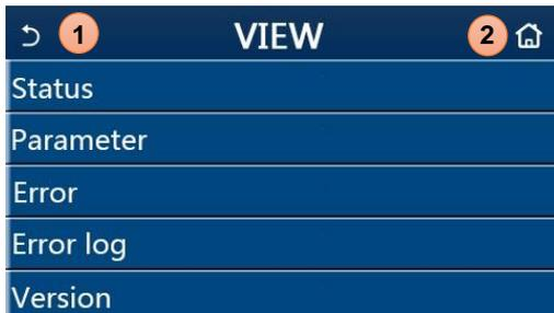
Through this menu it will be possible to view a lot of information relating to the operation of the machine; each label groups a set of information from which the user can check the status of the unit and any errors or anomalies in progress. To navigate in this menu, the system provides the following keys:
