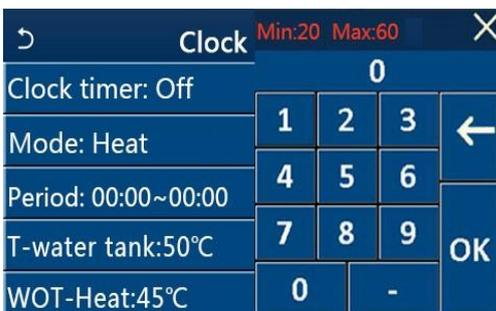
By clicking on the "Period" label, the page with the labels relating to the start and end times of the Timer will open; which will be set first by clicking on the label of the time you want to set, then sliding your finger over the time values until you select the desired ones; at the end, pressing the key at the top right will allow you to save the data entered.
